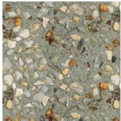
shared path_ washed aggregate concrete
