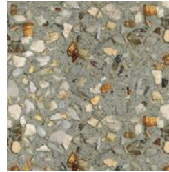
shared path_ washed aggregate concrete
