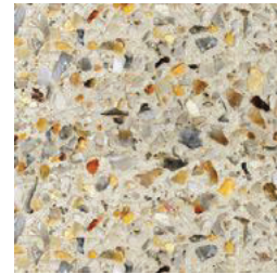
shared path_ washed aggregate concrete
