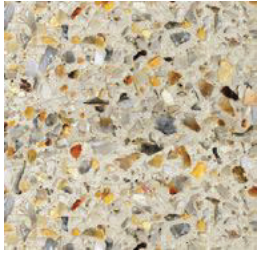
shared path_ washed aggregate concrete
