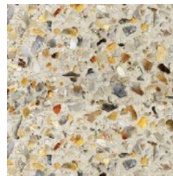
shared path_ washed aggregate concrete
