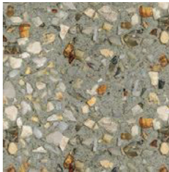
shared path_ washed aggregate concrete
