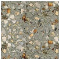
shared path_ washed aggregate concrete
