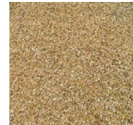
surface treatment_ stabilised gravel
