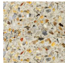
shared path_ washed aggregate concrete
