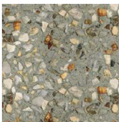
shared path_ washed aggregate concrete
