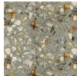
shared path_ washed aggregate concrete
