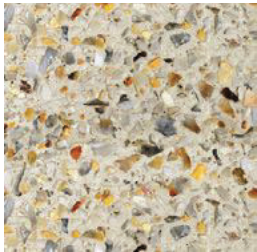
shared path_ washed aggregate concrete
