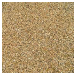
surface treatment_ stabilised gravel
