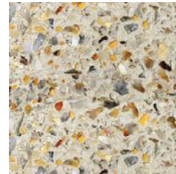
shared path_ washed aggregate concrete
